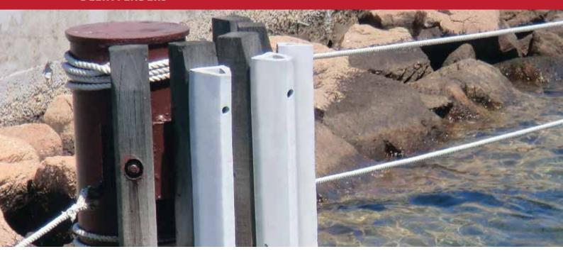
The delta fender is a proven effective rubber profile for use in both marine and industrial markets and they can be used for various purposes, both inside and outside. This type of fender has a minimal contact surface and they are easy to assemble. A properly mounted delta fender has the capacity to absorb high levels of energy through the presence of a relatively large hollow chamber.
