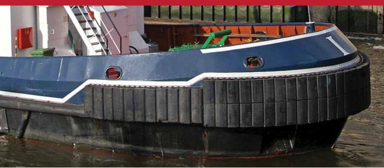
Keyhole fenders are used worldwide and they offer very reliable protection for the bow of a vessel or for the wall of a quay. This type of fender is characterised by the keyholeshaped opening on the inside and it is used in areas where large forces must be absorbed. Keyhole fenders are strong and they can be produced with a curve. The two mounting holes facilitate easy and accurate installation.
