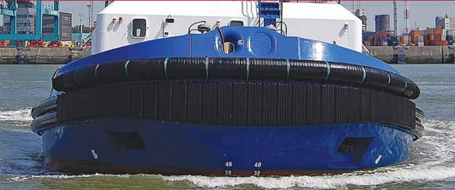
Cylindrical fenders on tugboats and workboats are often mounted on bow and stern mounted as the main push fenders. These fenders are often used on the bow in combination with Keyhole, M or W fenders. FenderTec produces this type of fender by means of a winding process up to a diameter of 1000 mm. If required they can be provided with tapered ends for better attachment to the ship and with grooves for additional attachment with chains or nylon straps.
